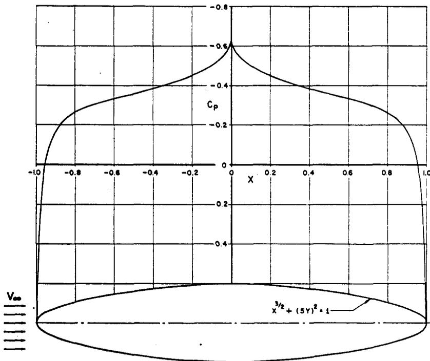
FIG. 64. Calculated pressure distribution on a two-dimensional body having zero curvature radius at the location of maximum thickness.
