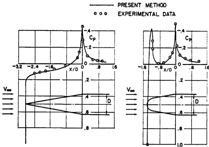
FIG. 42. Comparison of calculated and experimental pressure distributions on a pointed cone-cylinder and a blunted cone-cylinder.
