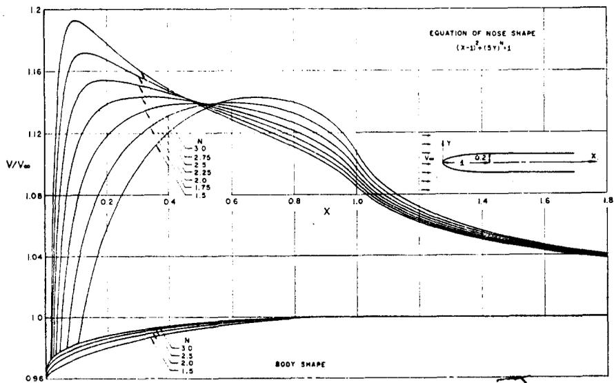
FIG. 63. Calculated velocity distributions on semi-infinite axisymmetric bodies with modified elliptical noses of 20 per cent semi-thickness.
