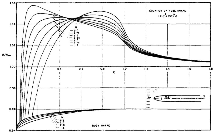
FIG. 62. Calculated velocity distributions on semi-infinite two-dimensional bodies with modified elliptical noses of 20 per cent semi-thickness.
