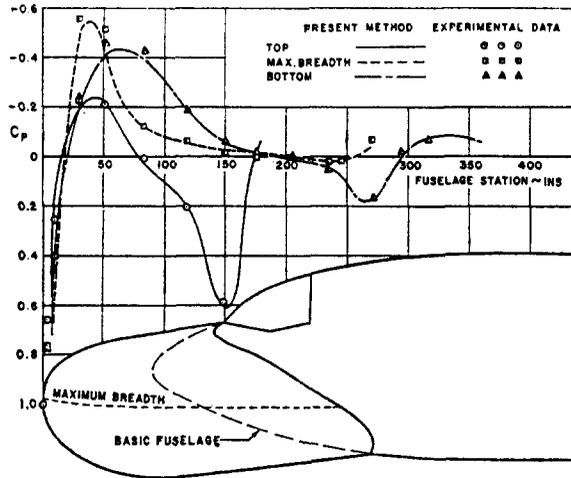
FIG. 51. Comparison of calculated and experimental pressure distributions on a C-135 fuselage with a large radome at zero angle of attack.
