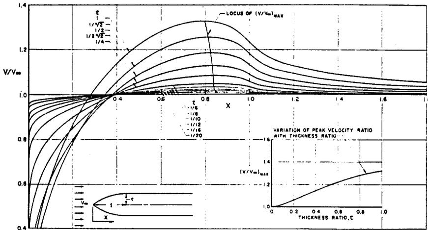
FIG. 61. Calculated velocity distributions on semi-infinite axisymmetric bodies with circular-arc noses.
