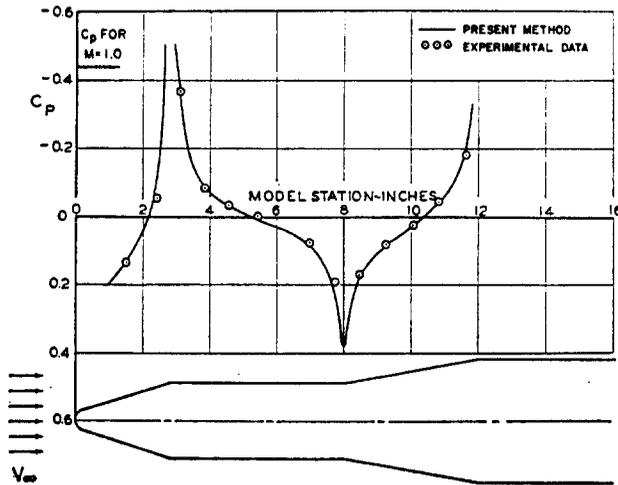
FIG. 45. Comparison of calculated and experimental pressure distributions on a Skybolt missile at a free-stream Mach number of 0.8.
