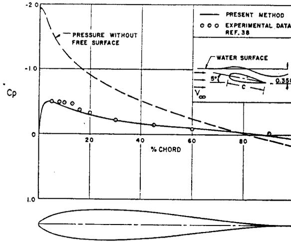
FIG. 39. Comparison of calculated and experimental pressure distributions on the upper surface of a 12 per cent thick symmetric Joukowski hydrofoil at 5° angle of attack, Froude number of 0.95, and a trailing-edge depth of 35 per cent chord. Also shown is the calculated pressure distribution without free-surface effect.
