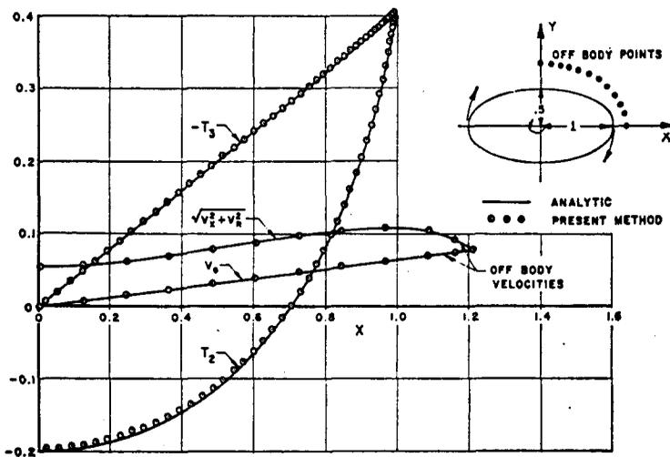
FIG. 33. Comparison of analytic and calculated velocity distributions on a prolate spheroid of thickness ratio 1/2 that is rotating about its center.
