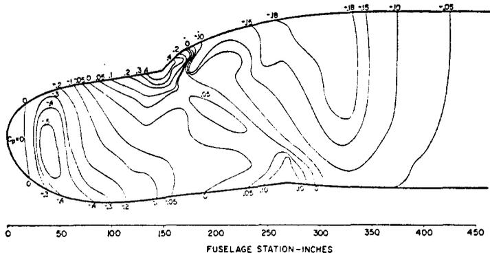
FIG. 52. Calculated isobars on a C-135 fuselage with a large radome at zero angle of attack.
