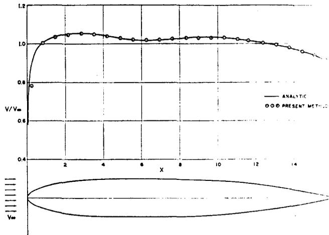
FIG. 29. Comparison of analytic and calculated velocity distributions on a source-sink body.
