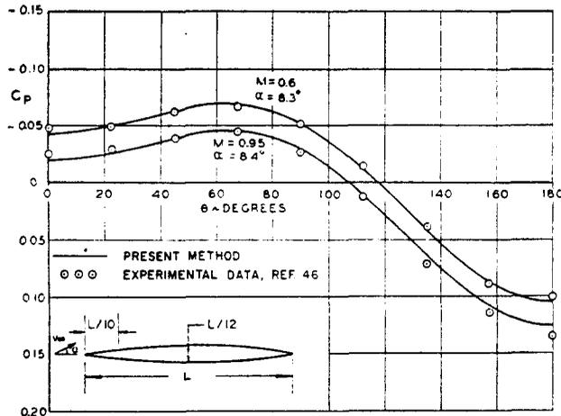
FIG. 49. Comparison of calculated and experimental circumferential pressure distributions at an axial location 0.1 of body length on a body at angle of attack for two high-subsonic free-stream Mach numbers.
