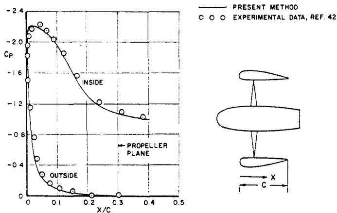
FIG. 43. Comparison of calculated and experimental pressure distributions on a propeller shroud with center-body in static operation.
