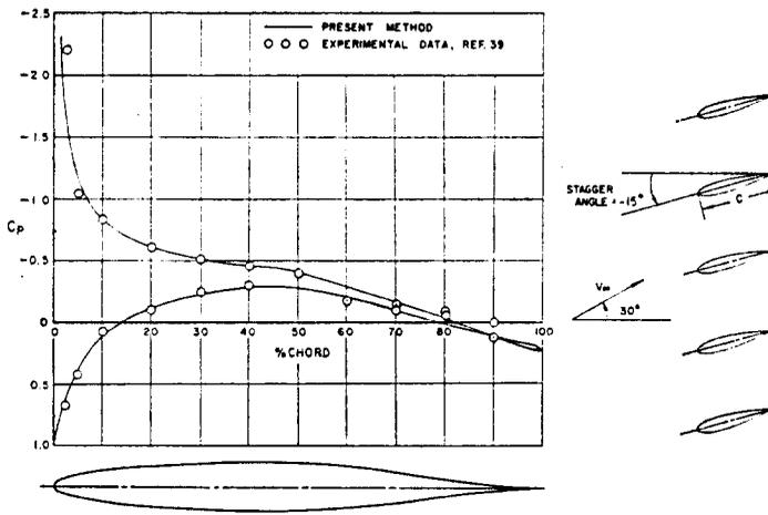
FIG. 40. Comparison of calculated and experimental pressure distributions on a symmetric NACA 65-010 airfoil in cascade at an inlet angle of 30° and a stagger angle of -15°.
