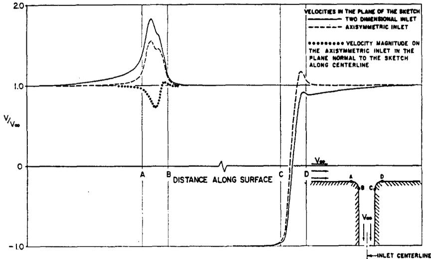
FIG. 67. Calculated velocity distributions on a two-dimensional and on an axisymmetric flush inlet for an inlet velocity equal to free-stream velocity.
