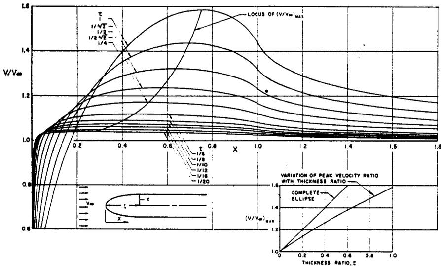
FIG. 58. Calculated velocity distributions on semi-infinite two-dimensional bodies with elliptical noses.
