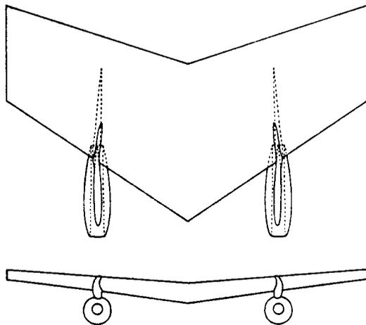
FIG. 56. Adjusted DC-8 wing-pylon-nacelle combination.
