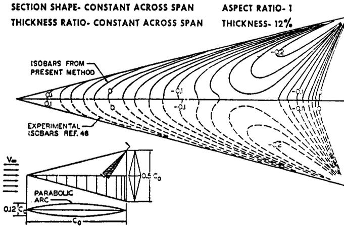
FIG. 53. Comparison of calculated and experimental isobars on a symmetric delta wing at zero lift.
