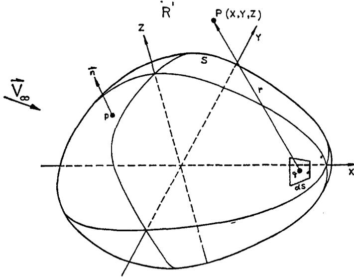
FIG. 1. Flow about a three-dimensional body surface.
