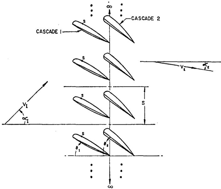
FIG. 17. Vector diagram showing inlet and exit velocities, angles, and some parameters.
