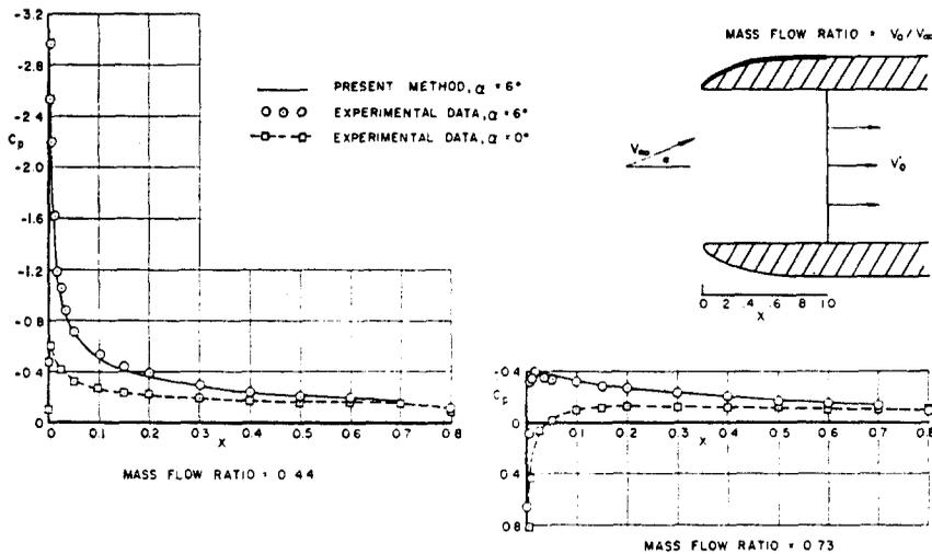
FIG. 47. Comparison of calculated and experimental pressure distributions on the exterior of an inlet lip at  $6^\circ$  angle of attack for two mass flow ratios.
