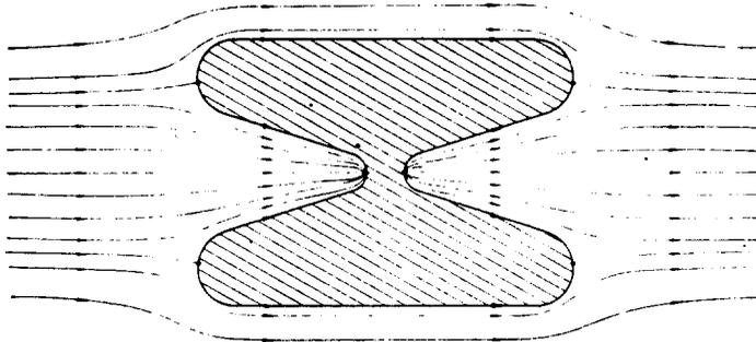
FIG. 65. Calculated streamlines in the plane containing the onset flow vector and the body's symmetry axis for uniform cross flow about an axisymmetric yo-yo type body.
