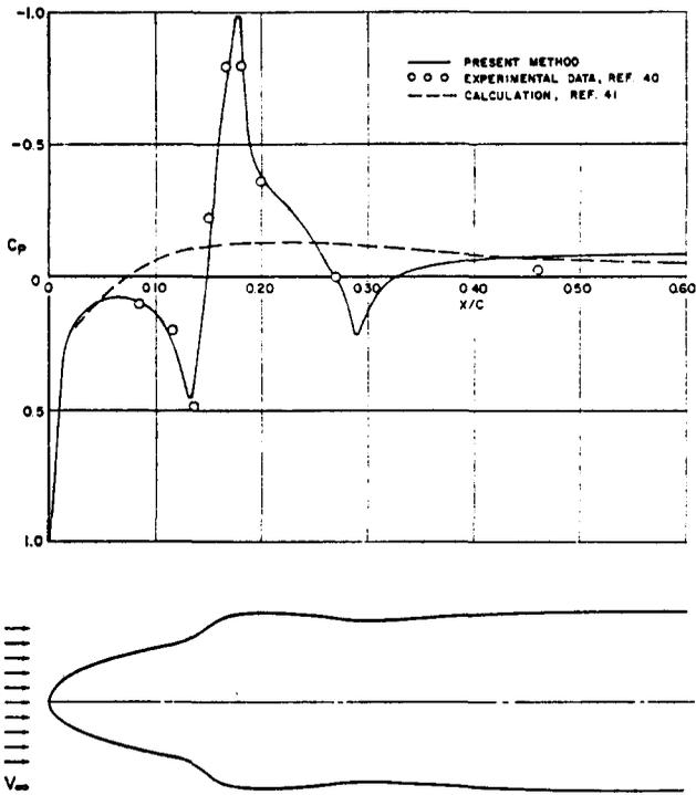
FIG. 41. Comparison of calculated and experimental pressure distributions on a prolate spheroid with an annular bump.
