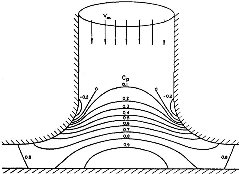
FIG. 66. Calculated isobars in a radial diffuser.
