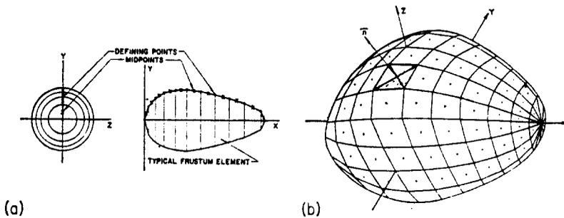
FIG. 3. Approximation of the body surface by elements. (a) Two-dimensional and axisymmetric bodies. (b) Three-dimensional bodies.
