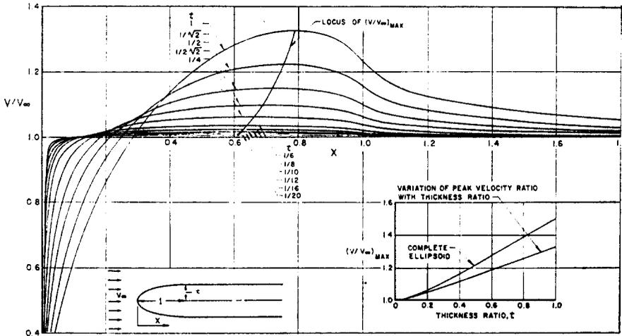
FIG. 59. Calculated velocity distributions on semi-infinite axisymmetric bodies with elliptical noses.
